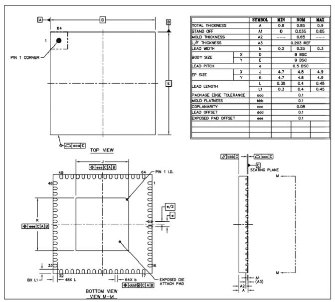
Figure 20 64-QFN Package Dimensions
