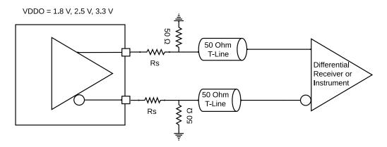
Figure 29 HCSL DC Coupled Termination. Source Terminated 50  $\Omega$
