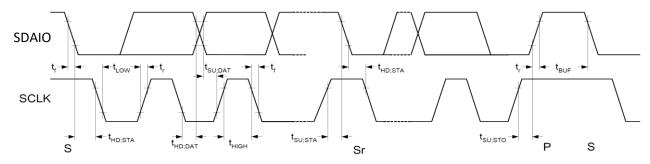
Figure 16 I2C Timing Waveform
