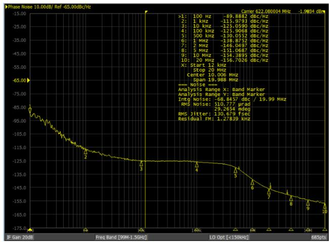
**Figure 3 Representative Phase Noise Measurement**
