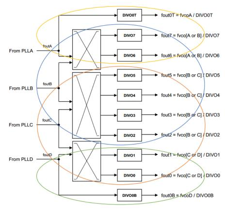
Figure 9 Output Clock Distribution
