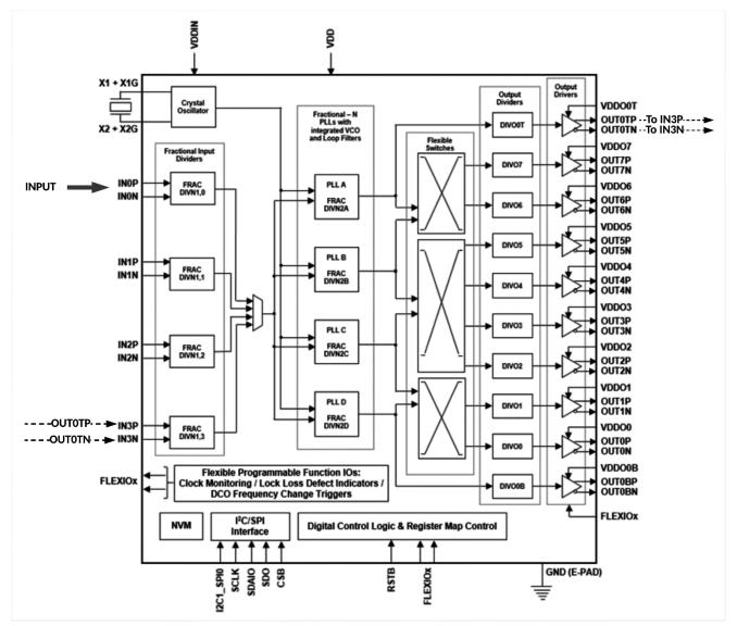
Figure 15 Zero Delay Mode Set Up: PLLA in ZDB mode with OUT0T routed in to IN3 for the ZDB feedback
