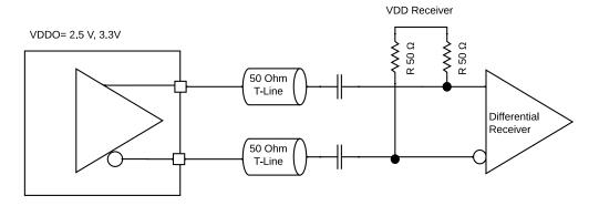
Figure 25 AC Coupled Receiver side resistive Termination options
