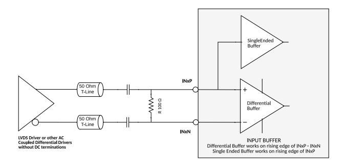
Figure 30 AC Coupled Differential LVDS Input / AC Coupled Driver without DC Terminations
