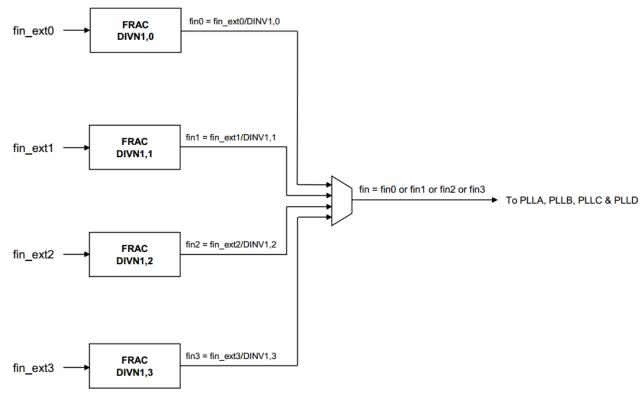
**Figure 7 Input Clock Distribution**
