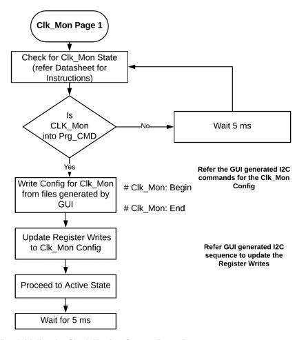
Figure 40 STEP 3: Initialise the Clock Monitor System Page- Page 1.
