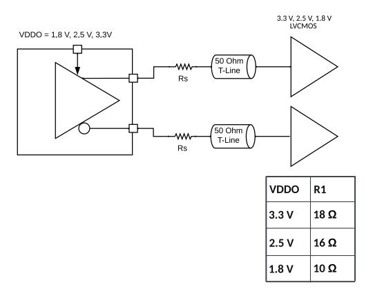
Figure 27 DC Coupled LVCMOS
