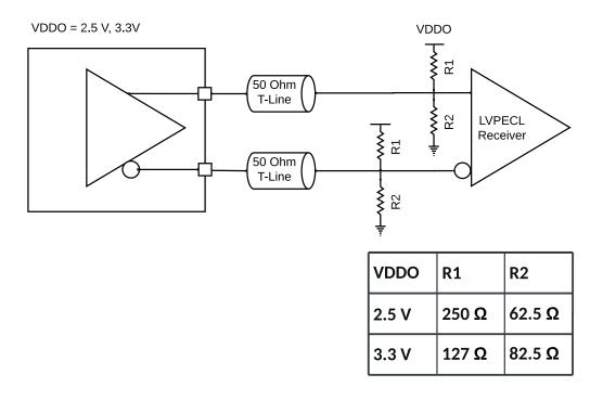
Figure 22 LVPECL Alternate DC Termination: Thevenin Equivalent
