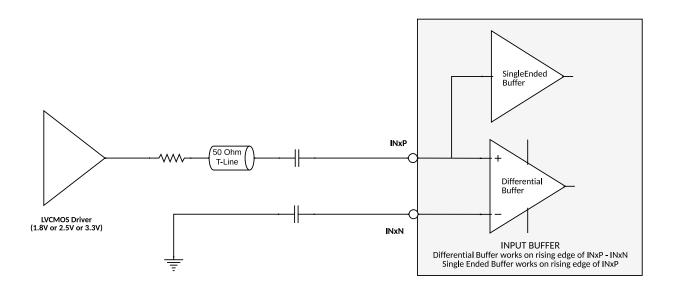
Figure 34 AC Coupled Single Ended LVCMOS input without 50 Ohm Termination
