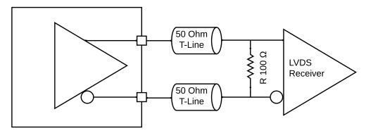
Figure 23 DC Coupled LVDS Termination
