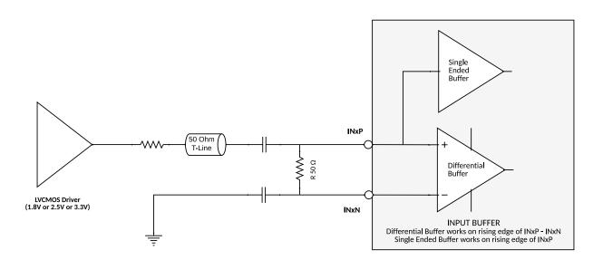
Figure 33 AC Coupled Single Ended Driver with 50 Ohm Termination on receiver (chip) side
