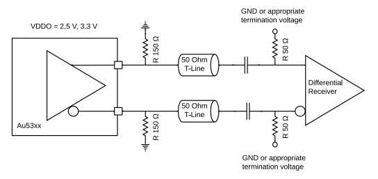
Figure 26 Alternate AC Coupled LVPECL with DC coupled resistors on Chip side
