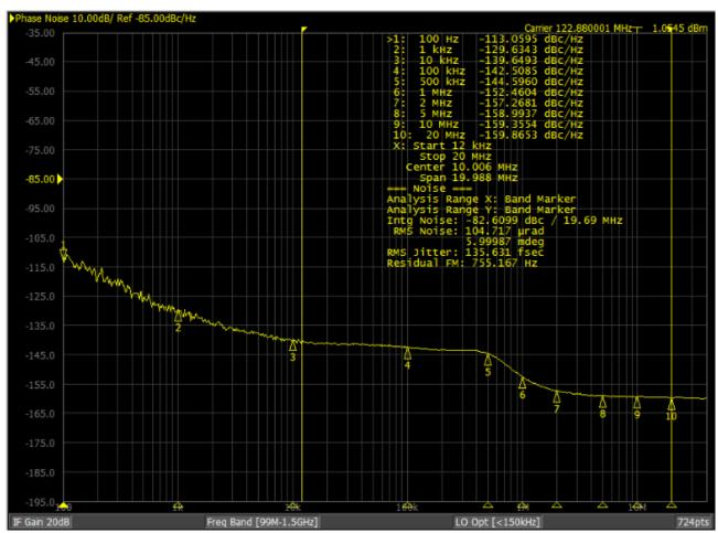
Figure 4 Representative Close In Phase Noise Measurement
