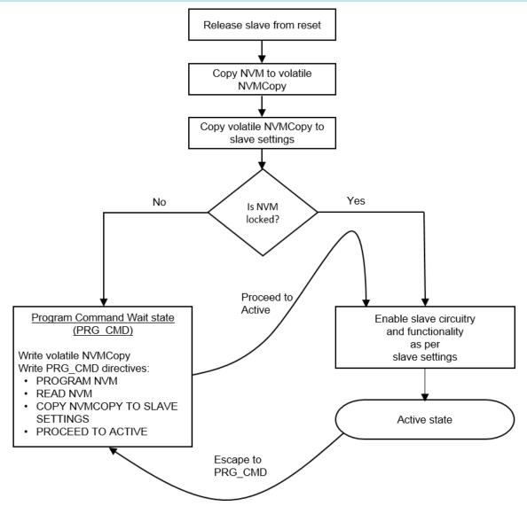
Figure 13 Slave Wake-up Finite State Machine
