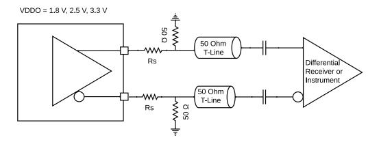
Figure 28 HCSL AC Coupled Termination. Source Terminated 50  $\Omega$
