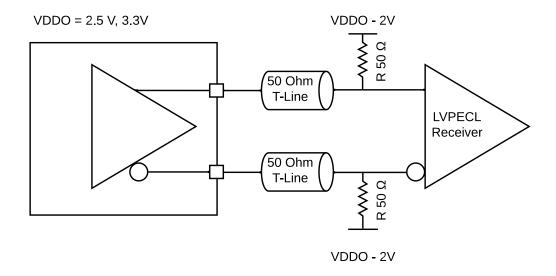
Figure 21 LVPECL DC Termination to VDDO - 2V
