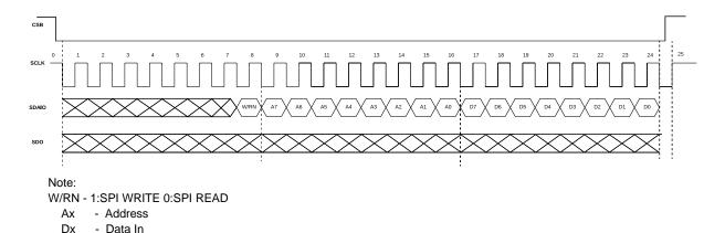
Figure 18 SPI Write
