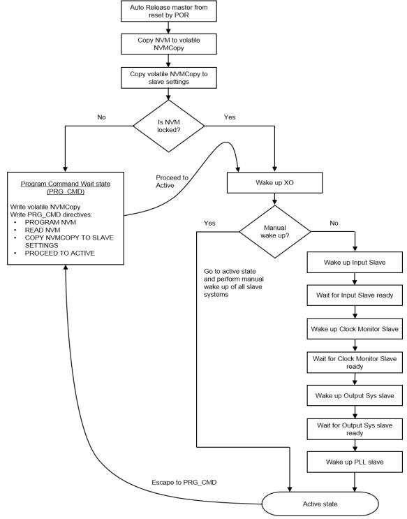
Figure 12 Master Wake-up Finite State Machine
