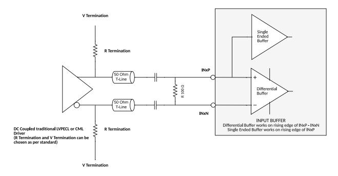
Figure 31 AC Coupled Differential LVPECL or CML
