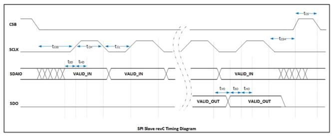
Figure 17 SPI Timing Diagram
